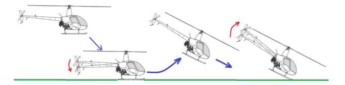
The helicopter after the flare had residual vertical and forward speed in excess.
