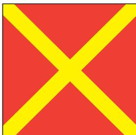
A red panel square with yellow stripes along each diagonal signifies that the aerodrome is unsafe for the movement of aircraft and that landing is prohibited.
