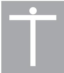
A white disc displayed alongside the cross arm of the T in line with the shaft of the T signifies that the direction of landing and take-off do not necessarily coincide.
