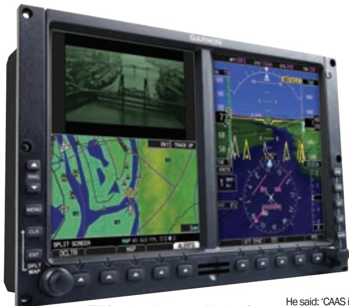
**EVS input can be seen on the Garmin G500 display. (Photos: Garmin)**
