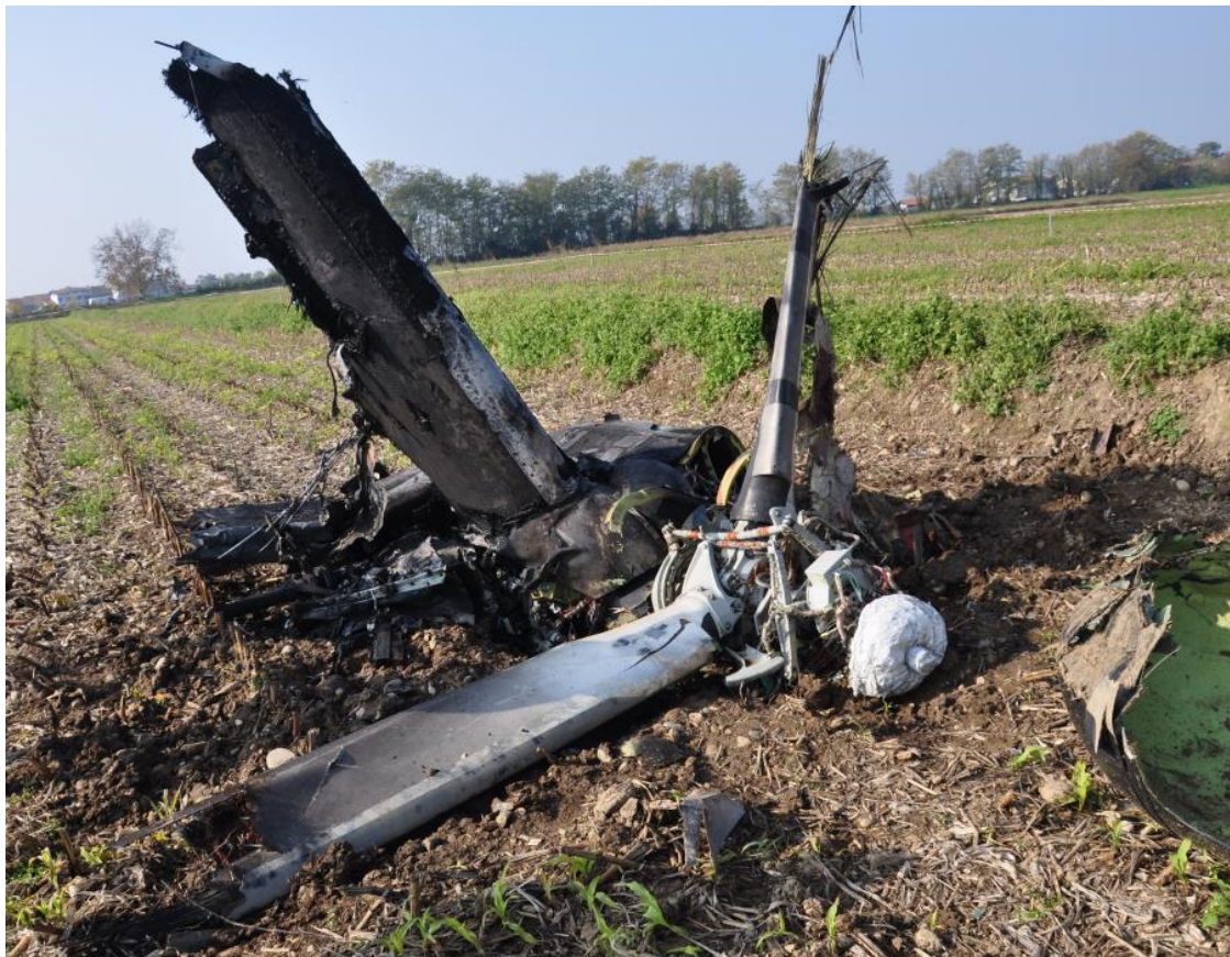
Photo 5: nacelle and parts of the right wing of the aircraft.
