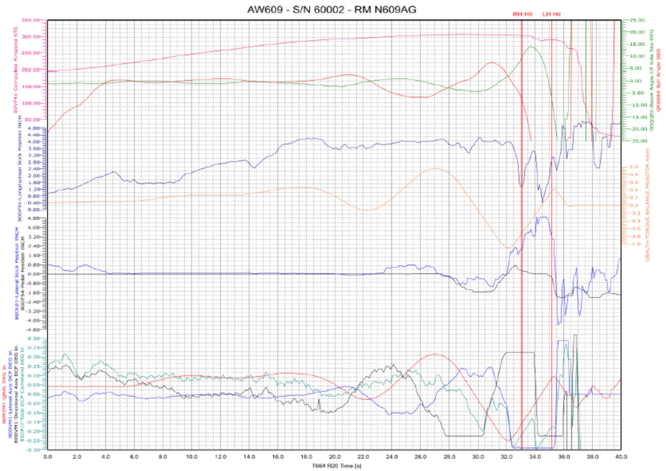
Figure 19: FTI data regarding flight mechanics and input from the pilot.
