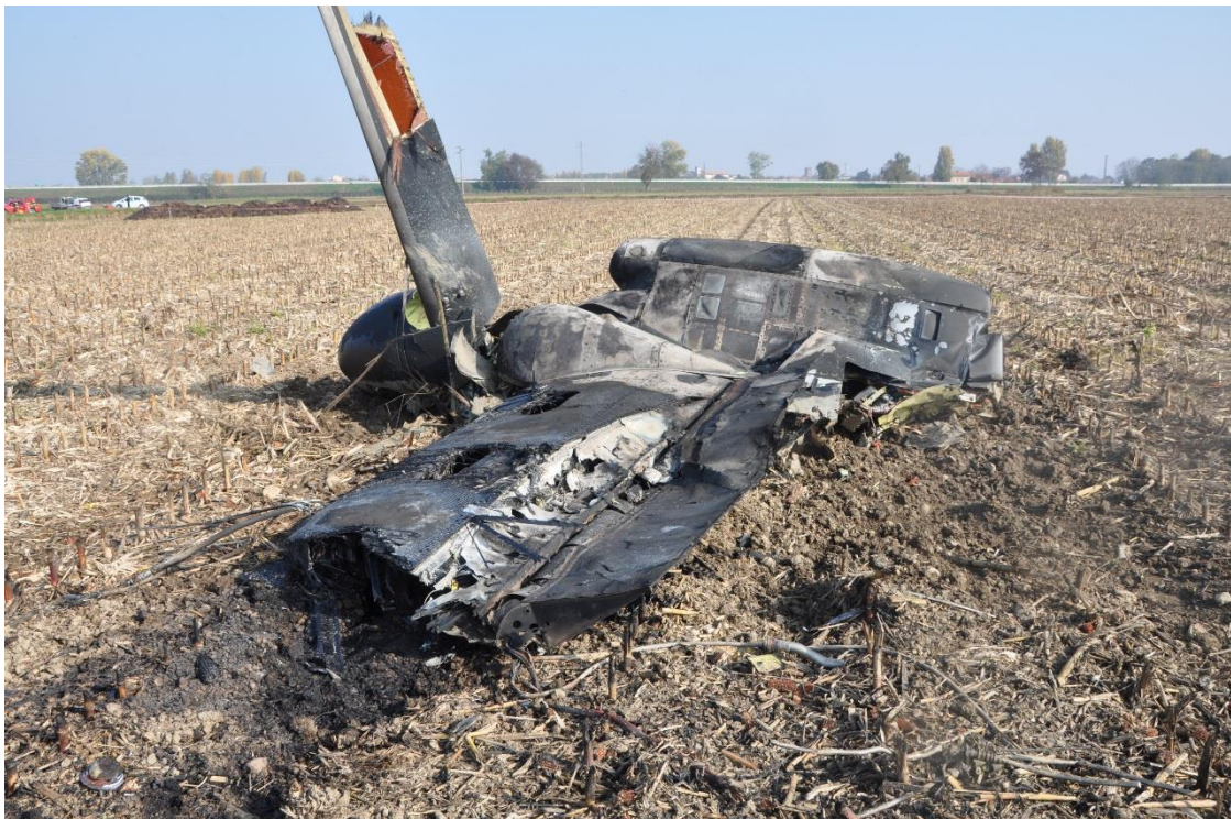
Photo 4: nacelle and parts of the left wing of the aircraft.
