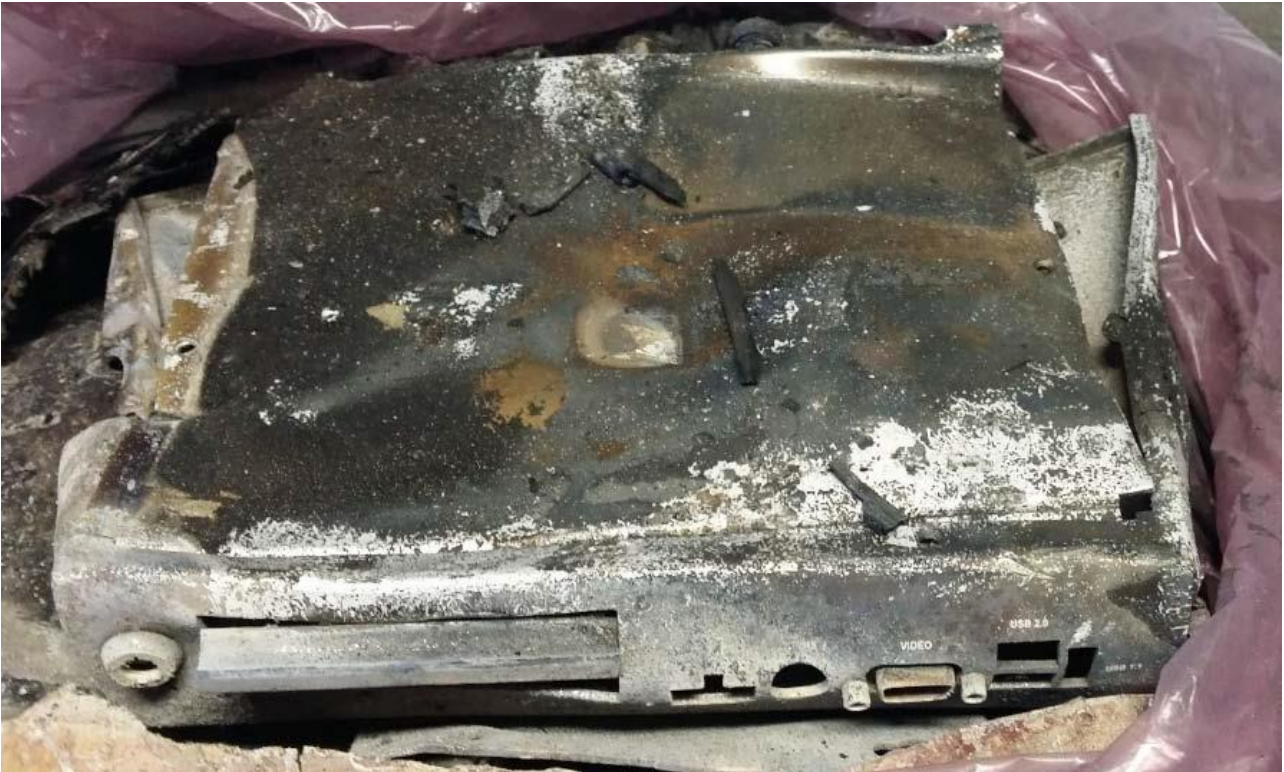
Photo 6: DVR system present on the aircraft.
