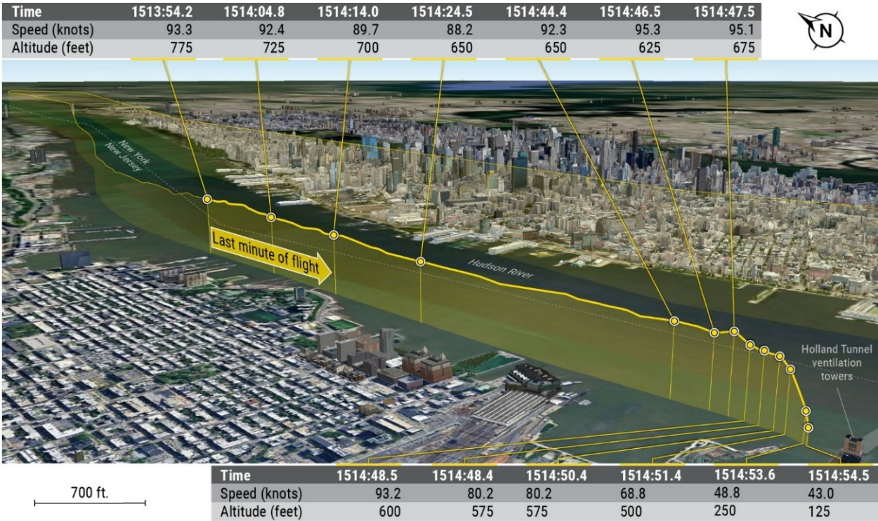
Figure 2. ADS-B flight track and geographic data highlighting the last minute of the flight through breakup, uncontrolled decent and loss of signal.
